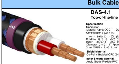
DAS-4.1 Top-of-the-line bulk balanced cable Specification Conductor Material Alpha-OCC + -DUCC (7N Class) Construction (pcs / mm) Inner - 59/0.13 -OCC (Right rotate) Middle- 29/0.13 -OCC (Right rotate) Outer- 36/0.13 -DUCC (Right rotate) Diameter (mm) 1.67 Approx. Size 15AWG / 1.65 Sq.mm Shield Material Cu-Foil + Braided OFC (24x6 / 0.13 α- OCC) +Paper wrap Inner Sheath Material Audio Grade Flexible PVC (Black) Nano-Ceramic / Carbon particle compound Diameter (mm) 7.80 Outer Sheath Material
